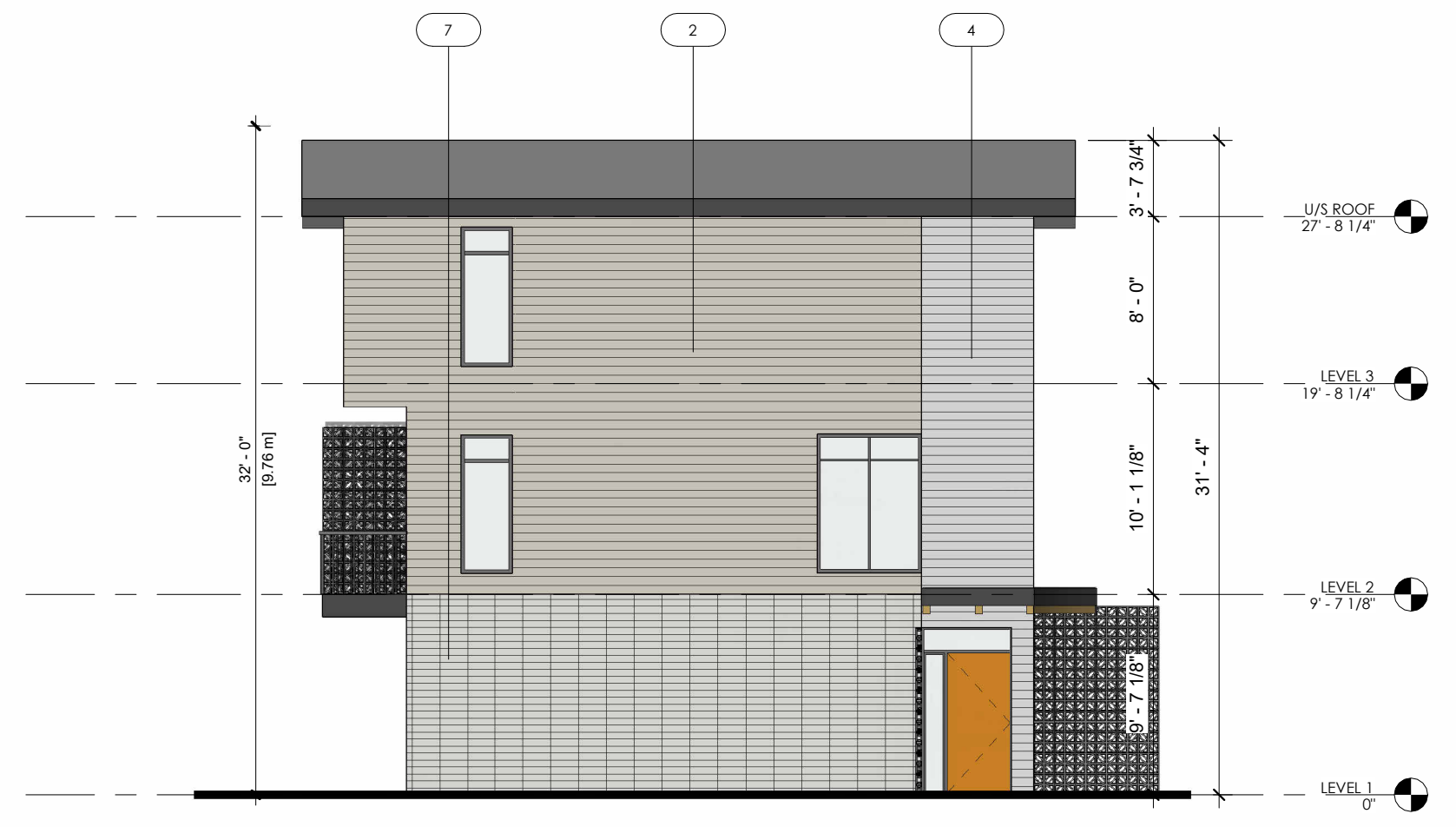
4 SOUTH ELEVATION - BUILDING D A3.2 1/8" = 1'-0"
